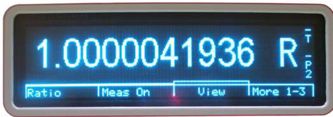
Examples of Actual 6622A Display Pictures Taken at Trade Shows - Note Std Dev is in ppm showing ppb performance!
