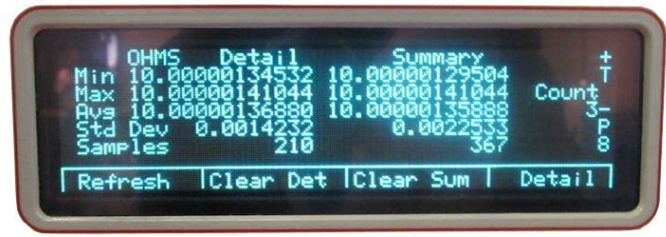
Examples of Actual 6622A Display Pictures Taken at Trade Shows - Note Std Dev is in ppm showing ppb performance!
